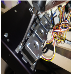
Loosen motor support bolts to reduce tension on belts. Do not remove
