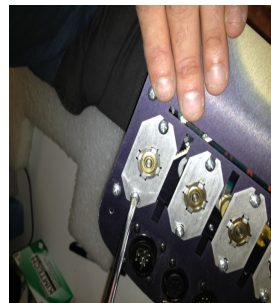
Belt tightening- Pull down on distal bearing side until the belt is tight (not too tight). Tighten bolts
